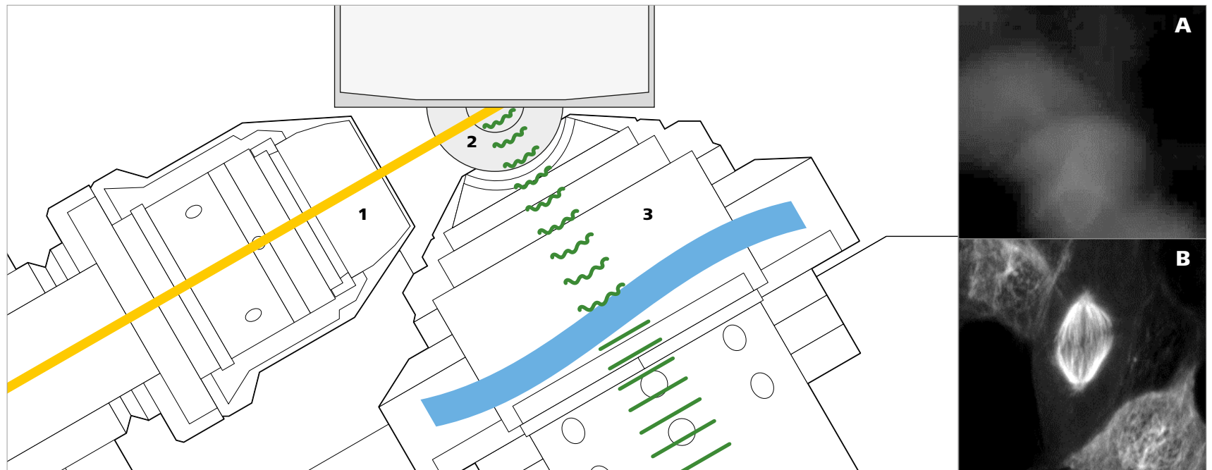
Schematic of sample carrier and core optics module with excitation objective (1), meniscus lens (2) and detection objective with free-form optics (3). Examples show imaging without (A) and with correction of refractive index changes (B).
