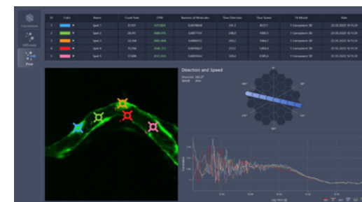
To determine the flow direction and speed within a liquid, a total of 27 detector element pairs are cross-correlated along 3 different axes of the Airyscan detector.
