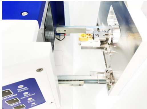
The cryo sample holder is transferred at room temperature onto the cryo stage through the standard airlock from ZEISS.
