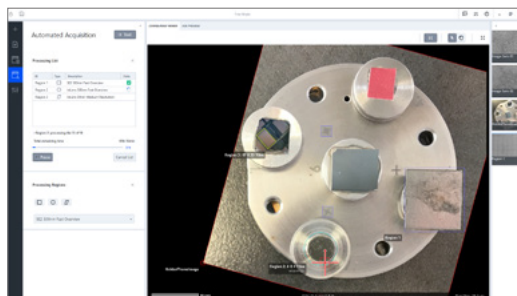
Create acquisition regions for SEM mosaics within the workspace from ZEN Connect and have them automatically acquired.
