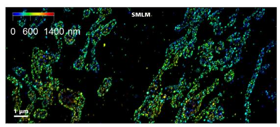
3D PAINT image of mitochondrial membranes in BSC1 (kidney epithelial cells). The outer membrane protein Tomm20 was labeled using Ultivue – I2-650 imaging strand. Reshaped PSF encoding for Z information was used to create a 1.4 µm deep 3D PAINT image. Upper figures show the widefield microscopy image (left) of the area as well as the 3D image of the modified PSF (right) used for 3D SMLM. Objective: alpha Plan-Apochromat 63×/1.46 Oil
