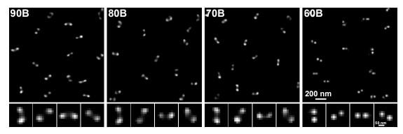
GATTA-STED Nanoruler 90B, 80B, 70B and 60B (GATTAquant, Germany) were imaged and processed with Elyra 7 Lattice SIM $^2$  mode with a 63×/1.4 oil objective. Distances of 90 nm, 80 nm, 70 nm and 60 nm are resolved.
