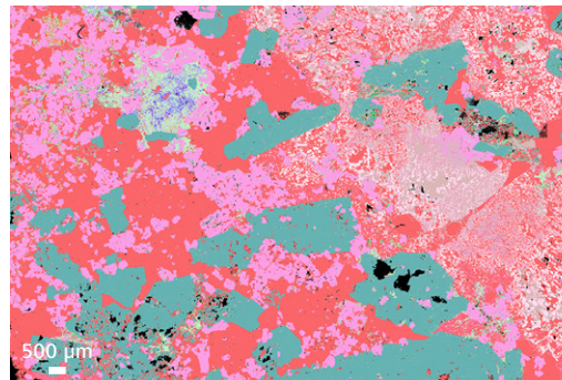
Peralkaline Granite, Northern Quebec, Canada, containing rare earth elements, including a fluorite vein that crosscuts the sample and zoned zircons.
