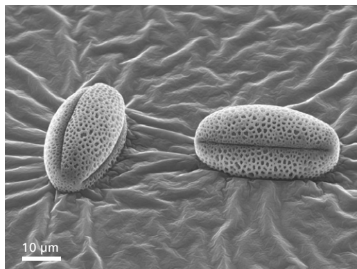
Freeze-dried pollen imaged at high vacuum conditions; SE detector, 10 kV
