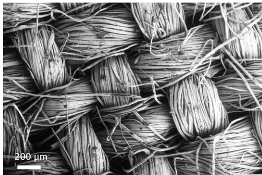
The C2D produces excellent images of uncoated samples in variable pressure mode, perfectly suited to forensic fiber comparisons.
